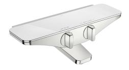
Thermostatic bath and shower faucet with easy-to-use control handles. Temperature limiter in the handle. Spacious shelf made of safety glass. The faucet is equipped with eccentric unions with silencer, litter filters and non-return valves.
